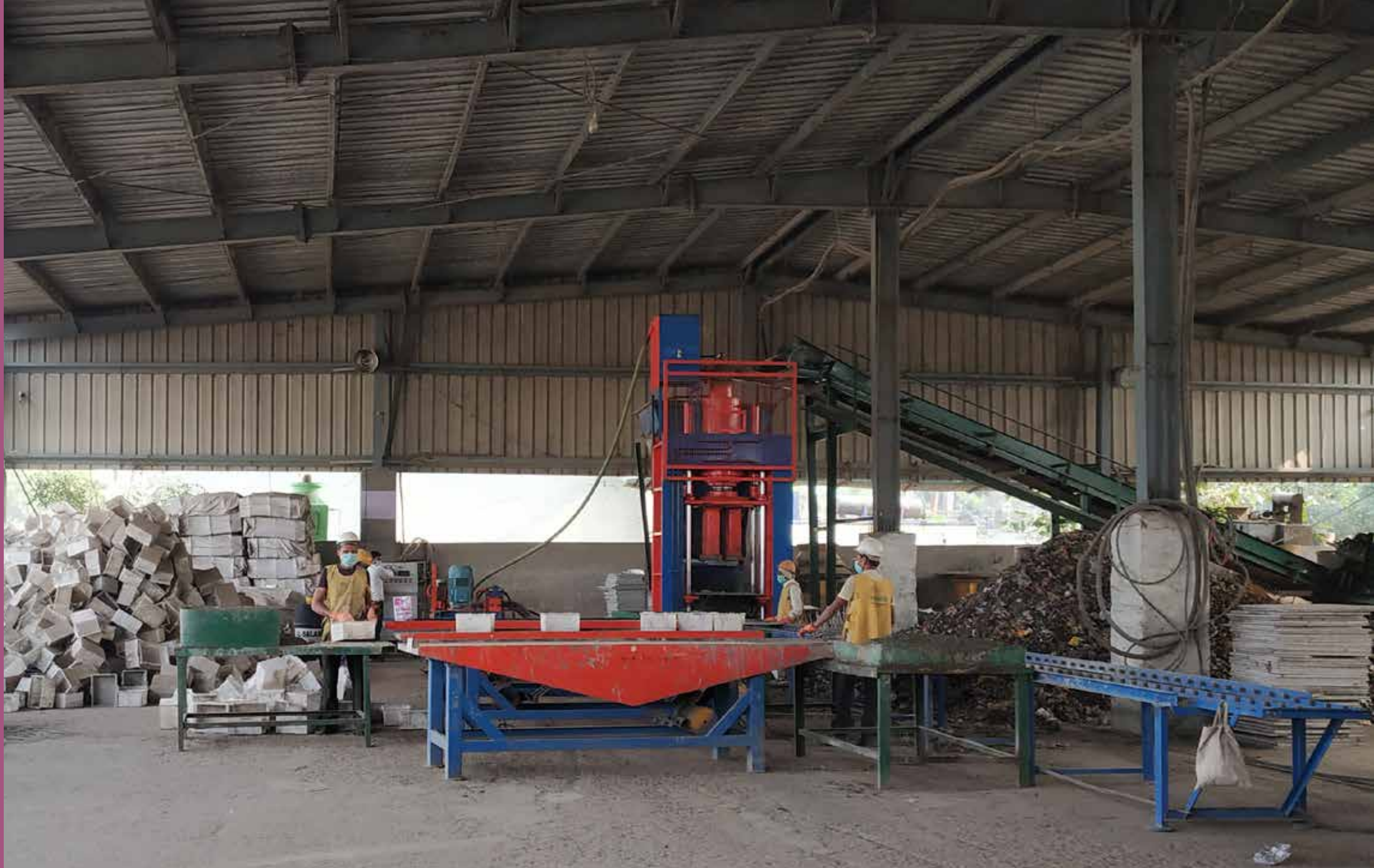
Dry Waste Compressed to make RDF Block
