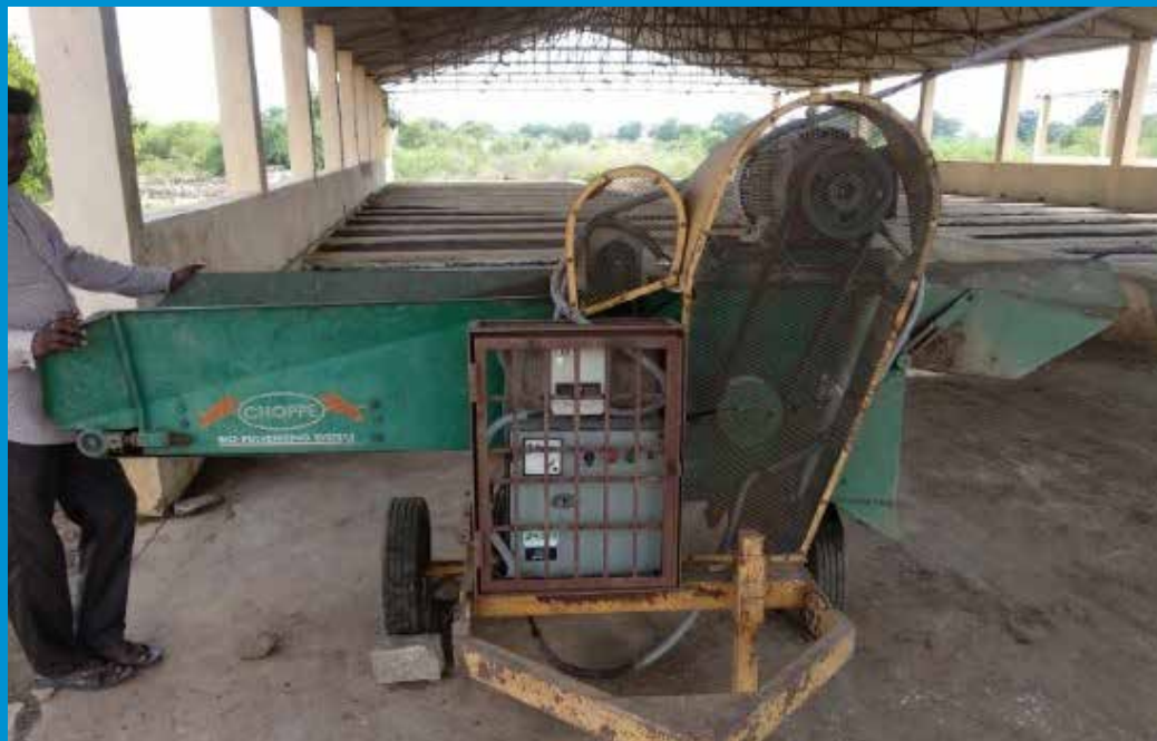
Shredding of Waste, Centralized Compost Plant
