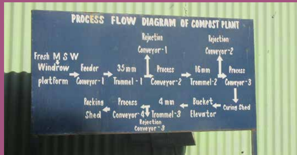
Process Flow Diagram of Compost Plant
